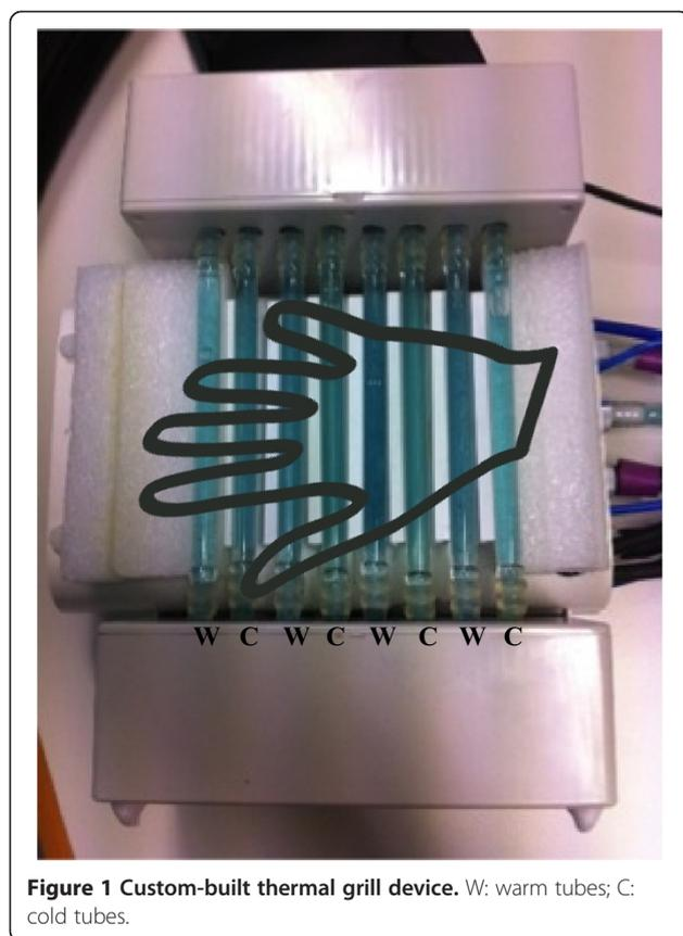
**Figure 1** Custom-built thermal grill device. W: warm tubes; C: cold tubes.
